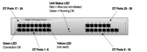
**Note:** The IP400 Digital Terminal 16 Expansion Module is only equipped with the bottom row of ports (1-16).
